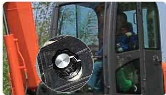
operator can easily switch attachments by turning on the switch in cab
