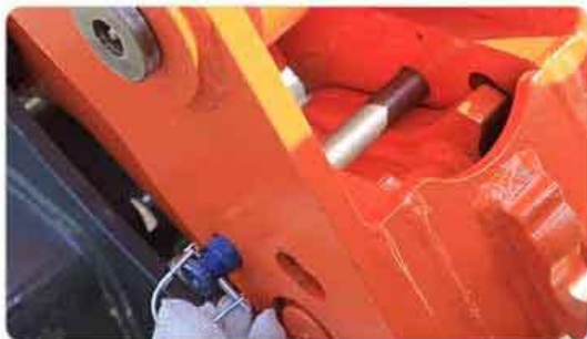
strong safety pin at accurate position
